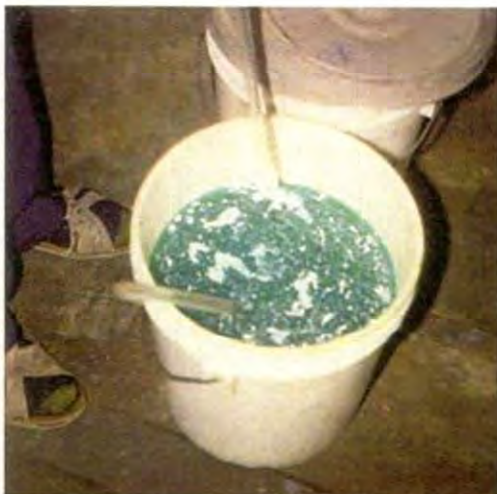
Figure 9: Addition of brine to silver nitrate solution.
