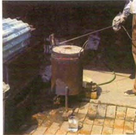
Figure 1: 'Homemade' gas furnace for melting silver and silver scrap.
