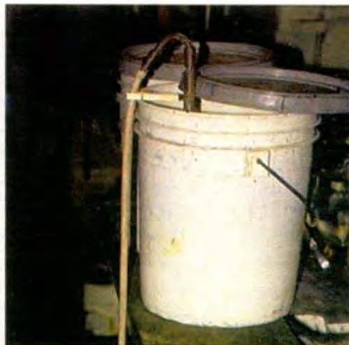
Figure 10: Addition of brine to silver nitrate solution near end of reaction.
