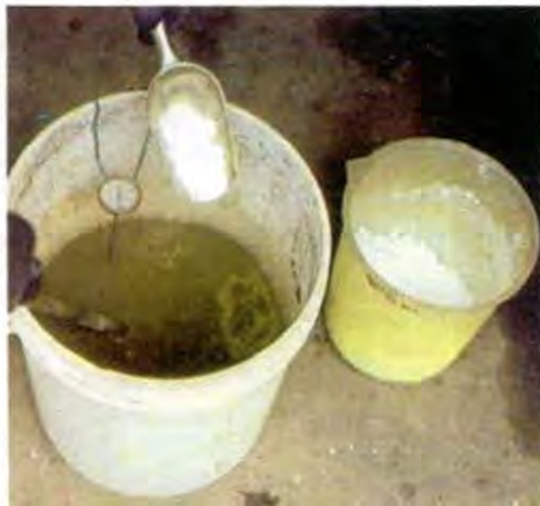
Figure 11: Precipitation of silver by addition of caustic soda to chloride/dextrose mixture.
