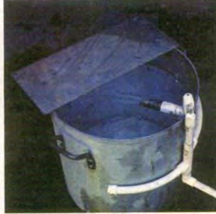
Figure 2: Container for making silver shot.
