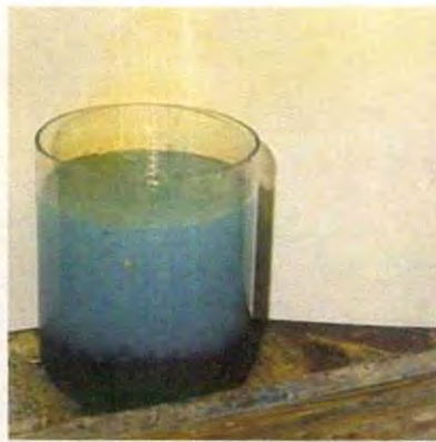
Figure 6: Dilute nitric acid dissolution of silver scrap.
