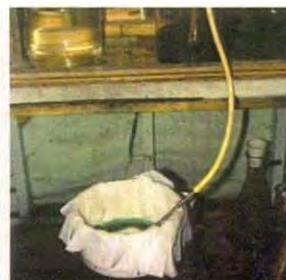
Figure 8: Suction filtration of silver nitrate through a Buchner funnel.
