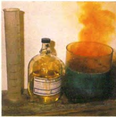
Figure 5: Reaction of strong nitric acid with silver shot.
