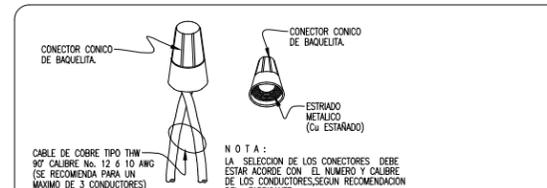
DETALLE TIPICO DE CONEXION PARA CONDUCTORES DE BAJA TENSION (220/127) CALIBRES No. 10 Y 12 AWG.
